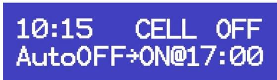
The first line of the display shows the current time and the cell status and output. In the example above the time is 10.15am and the Cell is “OFF”. If the Cell is on, the output of the Cell will be displayed. If the output of the Cell has been set at lower than 100%, “CELL OFF” will be displayed intermittently even while the unit is running as the Cell regulates output. (See Chlorine Output Menu on page 16 for more details)
