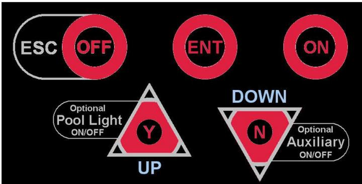
Each button is labelled with its primary function either on the button itself, or adjacent to it. Secondary functions are labelled within a curved white outline next to the relevant button. The buttons are backlit to show which are active at any given time, although the ESC/OFF button is always available to take you back to the home screen.
